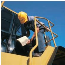
**Filter Access.** The left platform offers access to the primary filter, while the engine oil filter is accessed from the right platform.
