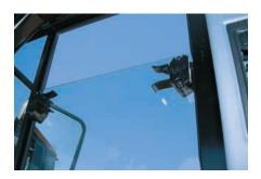
**Optional Sliding Cab Window.** Located in the right and left doors are optionals sliding windows to provide access to outside air without opening the door.
