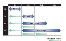
automatically downshifts from second to first when beginning the digging cycle. It automatically upshifts from first to second when the direction control lever is placed in reverse. This results in increased rim pull for better bucket penetration and reduced cycle times for higher productivity.
