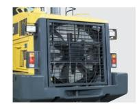
If the machine is operating in adverse conditions, the operator can reverse the hydraulic cooling fan from inside the cab by turning a switch on the control panel.
