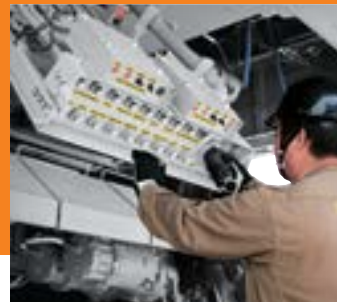
■ The auto-lubrication system for the front joint pins and swing circle saves service time.
