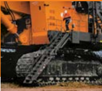
■ Folding stairs with wide steps allow for easy accessibility, servicing and maintenance.
