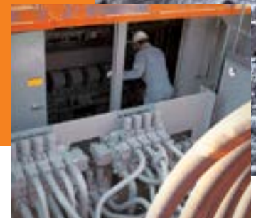
■ Located at the center of the machine, a wide-open service area gives you access to the engine as well as hydraulic and electrical systems.
