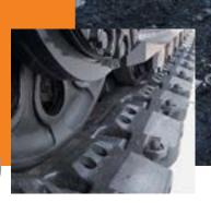
Rugged track links include roller guides to help extend service life.
