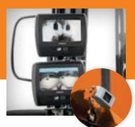
Four optional outside cameras can be mounted around the machine for enhanced visibility and help eliminate blind spots.
