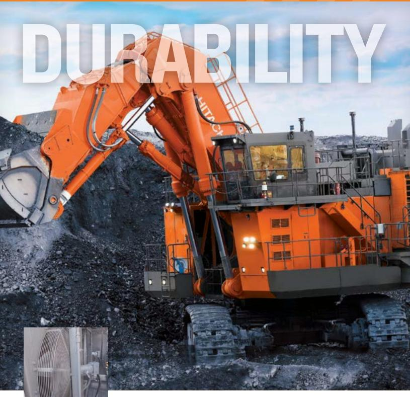
Four oil coolers are strategically positioned far from the engine radiator for even better cooling potential. With constant correct track tension, travel is automatically stopped if the nitrogen gas accumulator pressure exceeds a preset level. Alert information and countermeasures are indicated on the multi-display LCD monitor.
