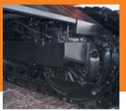
High-mounted compact travel motors are protected from rock damage. Optional travel motor guards provide an even higher level of protection from damage.
