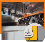
The cast steel structures, integrated into the center track frame, assist in avoiding stress concentration and increase reliability.
