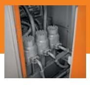
■ The centralized filter system makes inspection and maintenance quicker and more convenient.
