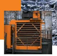
A walkway around the entire counterweight provides easy access to rear areas for faster, safer inspections and maintenance.
