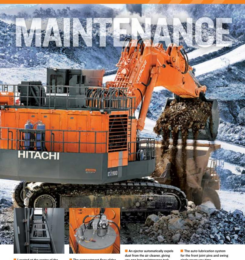
Located at the center of the machine, a wide-open service area gives you access to the engine as well as hydraulic and electrical systems.
