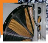
The oil cooler is strategically positioned far from the engine radiator for even better cooling potential.
