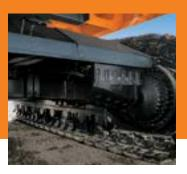
■ High-mounted compact travel motors are protected from rock damage. Optional travel motor guards provide an even higher level of protection from damage.
