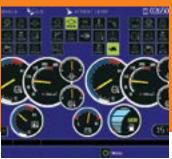
■ The multi-display, color LCD monitor provides machine data, operating status and alerts at a glance. The monitor can be preset to indicate replacement intervals for engine oil, hydraulic oil and filters.
