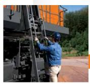
An optional slide ladder gives the operator even easier access to the cab and working platform.
