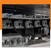
■ Track links are enlarged to increase strength for higher durability and reliability especially on rugged ground.
