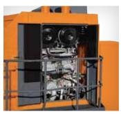
Auto Dust Ejector (Air Cleaner). The auto dust ejector automatically ejects airborne dust and particles to keep filter elements clean and extend their replacement intervals.
