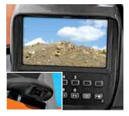
■ The standard remote rearview monitoring camera gives the operator wider vision of the work area, and eliminates almost all blind spots.
