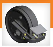
■ At the idler pedestal that sustains the front idler, its contact length is lengthened by approximately 90% to increase strength and service life.
