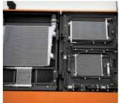
Parallel Arrangement of Radiator and Oil Cooler. The radiator and oil cooler are arranged side by side to increase cooling efficiency. This also reduces cleaning time and effort remarkably.
