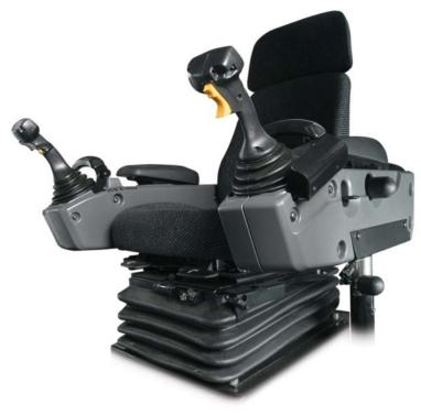
Operators are more comfortable and productive with two electro-hydraulic joysticks. New and experienced operators around the world report that the controls are easy to learn, and that the electronically adjustable control pods help position them for optimal comfort, visibility and proper operation.
